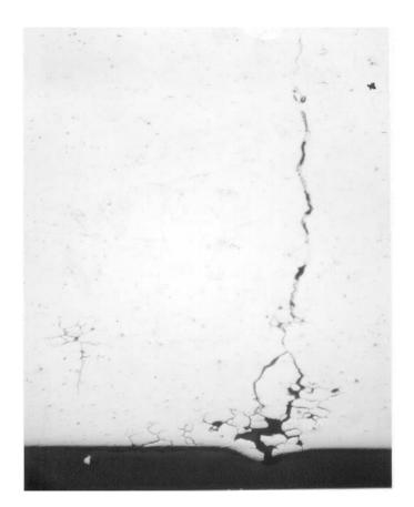
**Figure 1 – HW Cylinders (AA 6061)** Fatigue crack initiated from a corrosion pit. Magnification X 125
